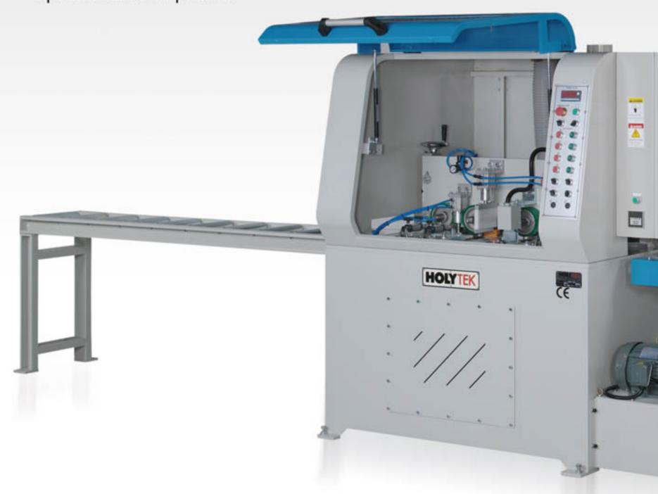
Holytek End Matching Machine with 2.5 long motorize infeed conveyor and 2.5m long idle outfeed roller or motorized conveyor (optional). The all-enclosed gua system ensures the safety of operators.
